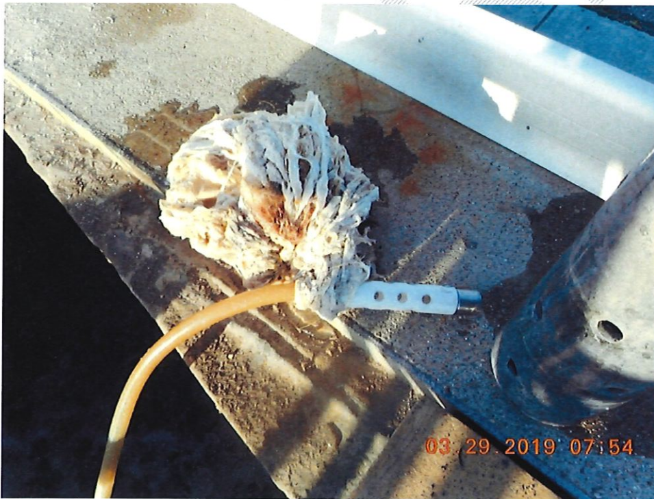
Figure 5-11 Rags Attached to Portable Sampler Intake Strainer on 3-29-19
